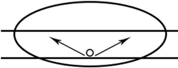
Type IV light distributions have a preferred lateral width of 60 degrees. This distribution is intended for side-of-road mounting and is generally used on wide roadways where the roadway width does not exceed 3.7 times the mounting height.
