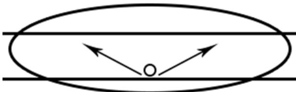
Type III light distributions have a preferred lateral width of 40 degrees. This distribution is intended for luminaires mounted at or near the side of medium width roadways or areas, where the width of the roadway or area does not exceed 2.75 times the mounting height.
