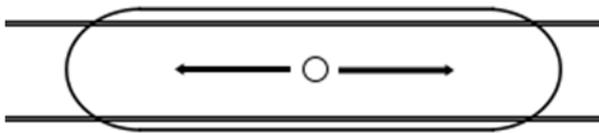
The Type I distribution is great for lighting walkways, paths and sidewalks. This type of lighting is meant to be placed near the center of the pathway. This provides adequate lighting for smaller pathways.
