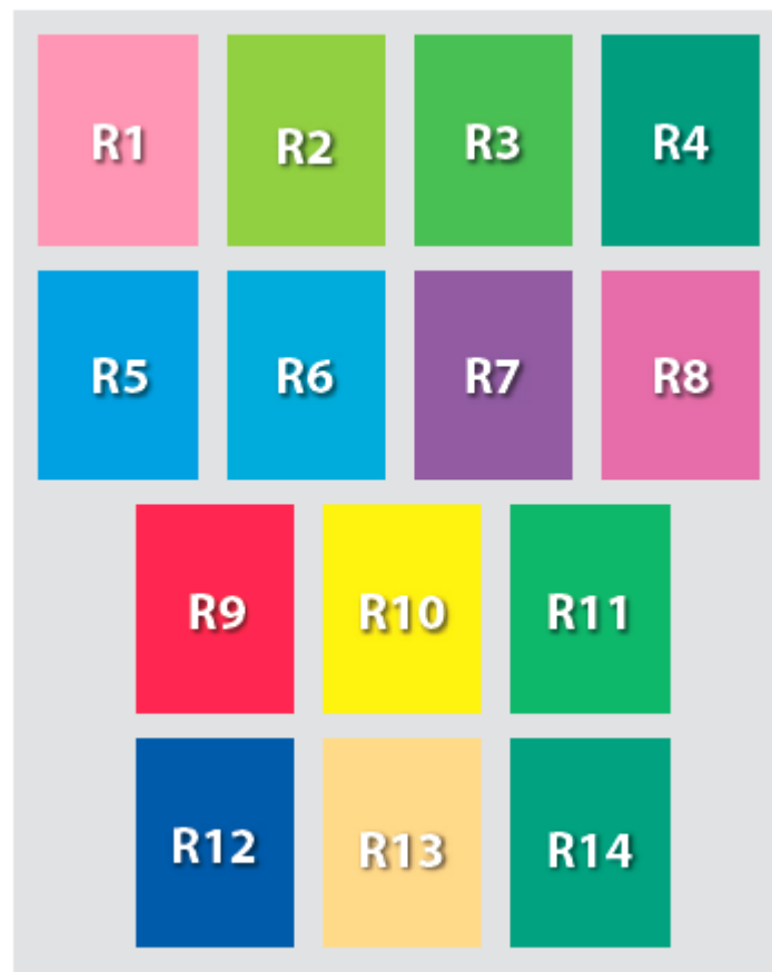
Test Colors Used In Calculating CRI
